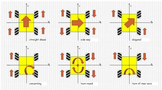
Fig-4: Net forces formed on Mecanum Wheels
