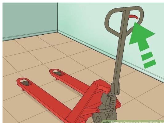
**Push inward on the drop lever to lower the legs.** If the legs are already completely lowered, you will not see them move. The legs should only be an inch or two from the floor.
