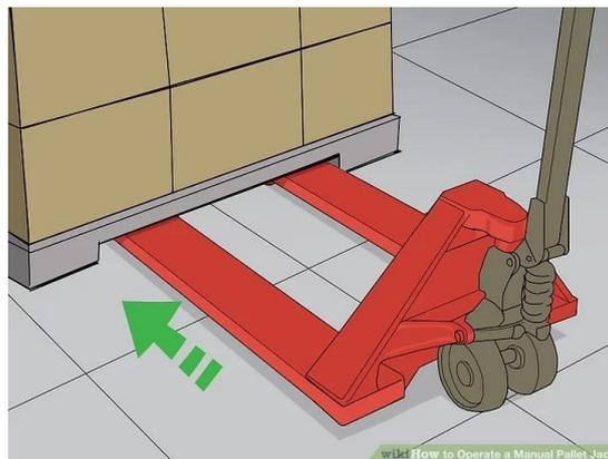
**Use the handle to jack up the pallet jack.** When the legs are under the skid, pull the vertical stem toward you, away from the pallet and toward the floor in a diagonal motion. You should feel the pallet truck (and the pallet) slowly rising against the pressure of gravity.
