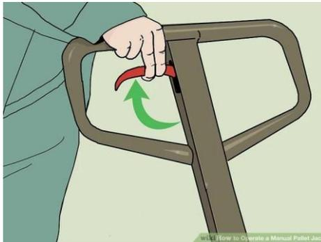
**Put the legs underneath the skid or pallet.** You will see when approaching the skid whether or not the product will fit underneath. If they will not fit, the machine has not been lowered sufficiently, so try to push again on the drop lever.
