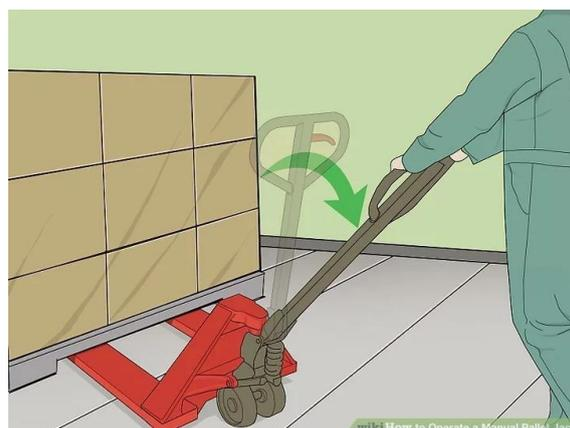
**Check to make sure that the pallet truck is not on the cross wood of the skid, front wheels must be on the floor.** If the wheels are on the cross wood this will stop the pallet from going up and also stop it from rolling.
