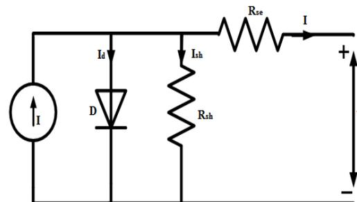
Fig: 2 Basic solar cell circuit
