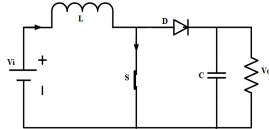
Fig: 4 Operation of Step-up Converter (Switch On)
