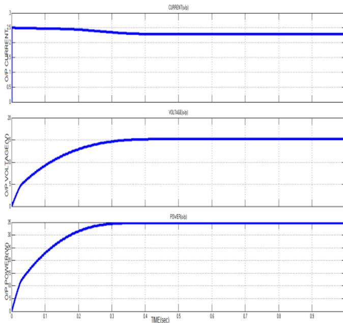
Fig: 10 Output current/voltage/power for P&O Controller
