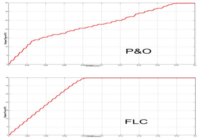
Fig: 13 Evaluation for Output Power of P&O and FL Controllers
