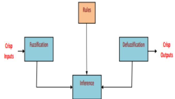
Fig: 7 Components of Fuzzy Logic Controller
