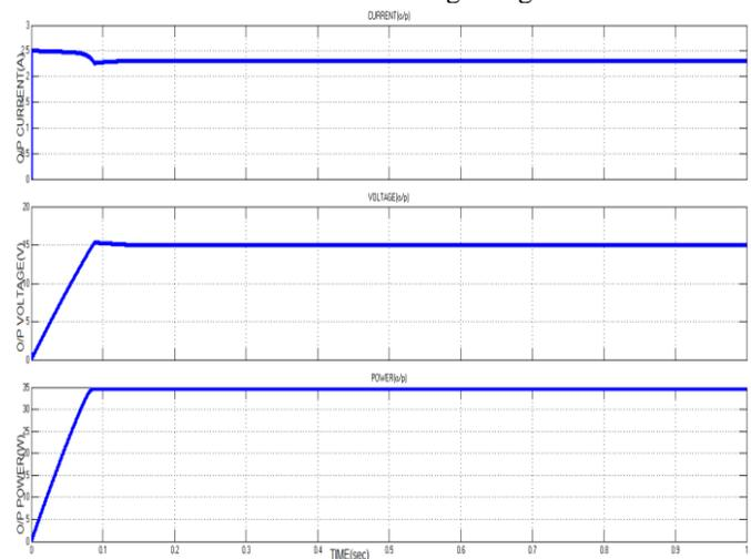
Fig: 12 Output current/voltage/power with FL Controller
