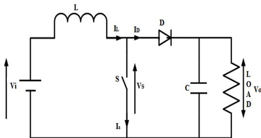
Fig: 3 Basic circuit of Step-up Converter
