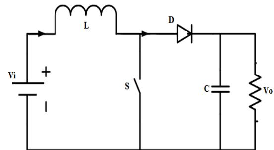
Fig: 5 Operation of Step-up Converter (Switch Off)
