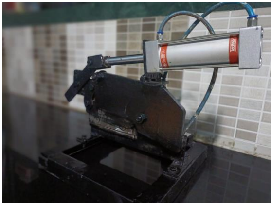
Fig. -2: Fabrication of Pneumatic Sheet Metal Cutting Machine
