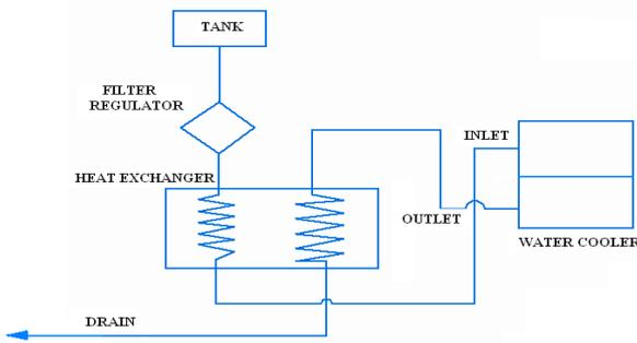
Fig 2: Block diagram of water cooler with heat-exchanger
