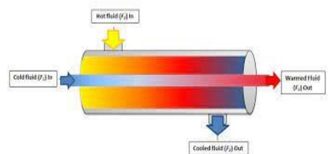
Fig 1: Block diagram of heat-exchanger
