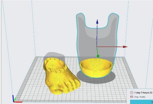
**Fig4.5: Layer by layer slices of uploaded foot & socket design STL file.**
