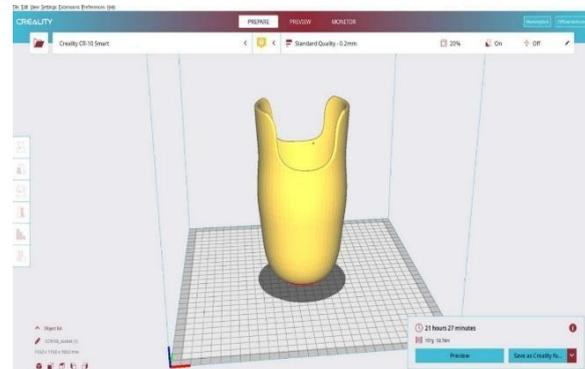
**Fig4.3:** uploaded socket design in slicer software.
