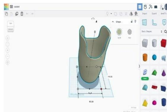
**Fig4.1:** Design output of socket in tinkercad design software.
