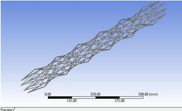
**Fig-7: Meshed Geometry of Isotruss Structure**
