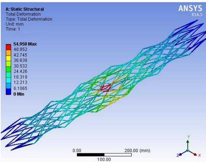
**Fig-8: Maximum deformation obtained in bending analysis**
