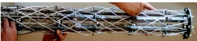
**Fig-15: Winding of Helical Members**
