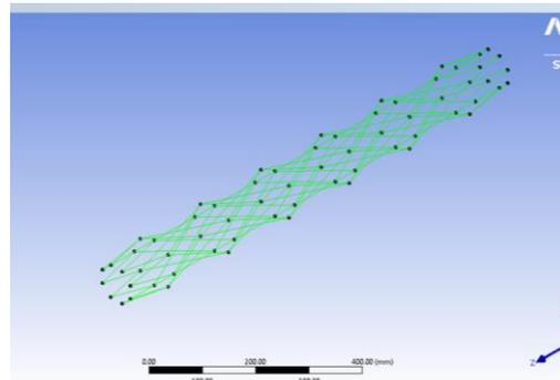
Fig-6: Final Isotruss Structure after joining of Node Points
