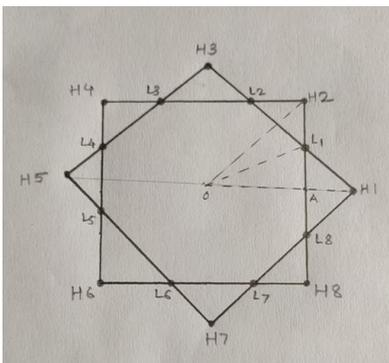
Fig-4: Top view of Isotruss Structure
