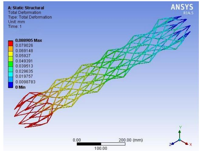
**Fig-9: Maximum deformation of G.I. wire Isotruss structure in compression analysis**
