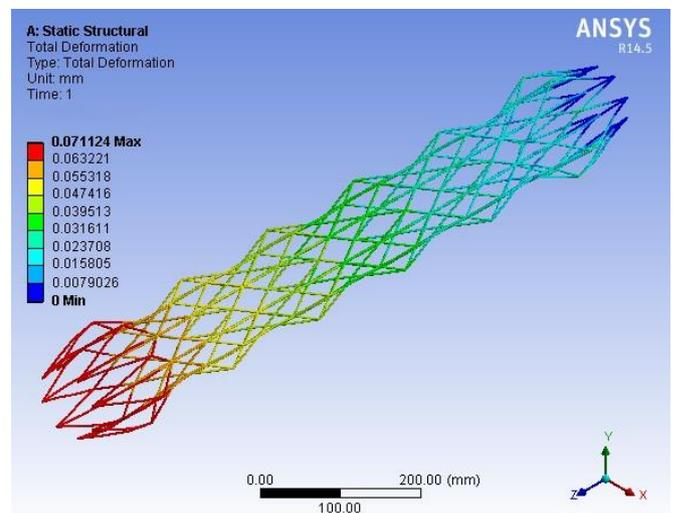
**Fig-10: Maximum deformation of carbon composite Isotruss structure in compression analysis.**
