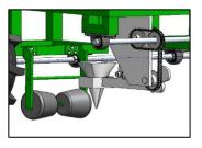
FIGURE.4.(C) DIGGING AND CLOSURE SYSTEM
