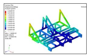
FIGURE.6.(B) LONGITUDINAL TORSIONAL DISPLACEMENT
