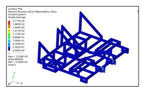
FIGURE.6.(C) VERTICAL BENDING STRESS
