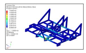
FIGURE.6.(E) TRANSVERSE BENDING STRESS
