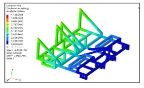
FIGURE.6.(D) VERTICAL BENDING DISPLACEMENT
