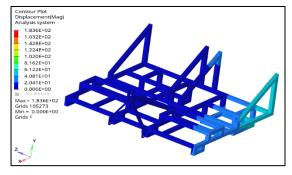
FIGURE6.(F) TRANSVERSE BENDING DISPLACEMENT
