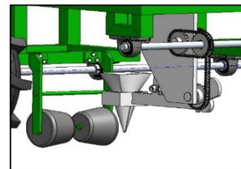
**FIGURE.4.(C) DIGGING AND CLOSURE SYSTEM**
