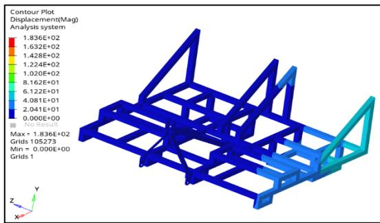
FIGURE6.(F) TRANSVERSE BENDING DISPLACEMENT
