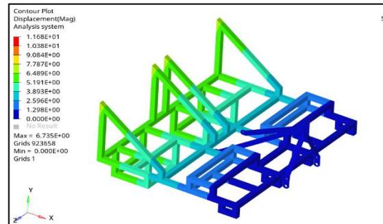
**FIGURE.6.(D) VERTICAL BENDING DISPLACEMENT**
