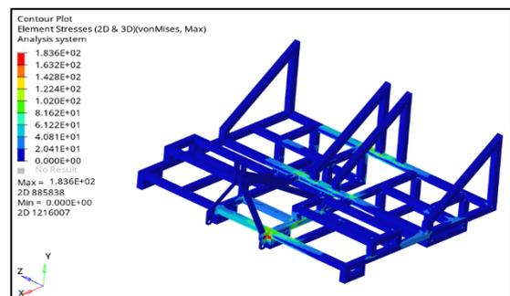
**FIGURE.6.(E) TRANSVERSE BENDING STRESS**
