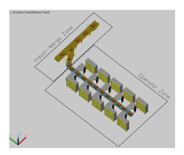
Figure -1: CAD model of Induct Merge Area
