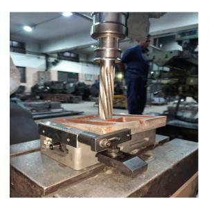
Thus the self-cantering vice has been manufactured successfully and drilling operation has been performed in the workpiece.
