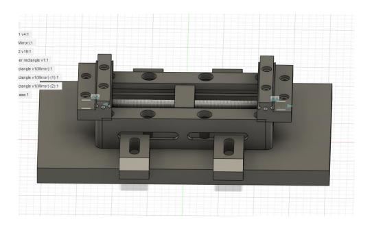
**Selection of Material (20mn Cr 5):** 20MnCr5 is a low-alloy steel that is commonly used in the manufacturing of vise bodies or bases. This is because it offers a number of properties that make it well-suited for this application.
