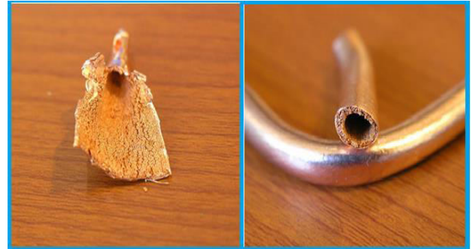
Fig: sintered metal powder wick
