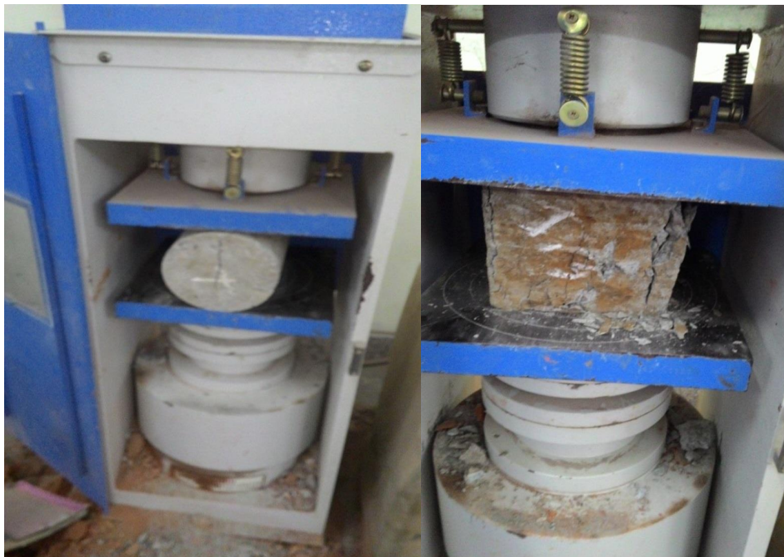
Figure 3: Testing of a cube on hydraulic testing machine
