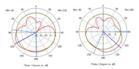
Fig 13.b-Radiation patterns at 8 GHz
