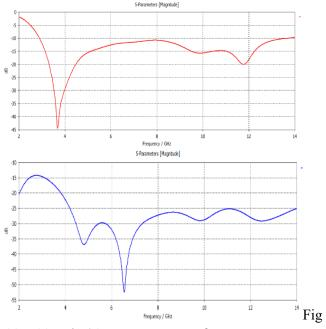
11. S11 and S21 Parameter Waveforms.
