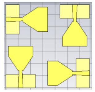
Fig 8.Schematic Diagram of Four Port UWB MIMOAntennawithoutstubs.
