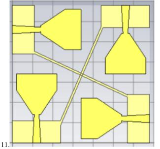
Fig 10.Schematic Diagram of Four Port UWB MIMO Antenna using Stubs.
