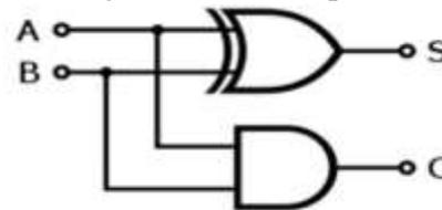
**Fig 3.1.1** Logical diagram of Half Adder
