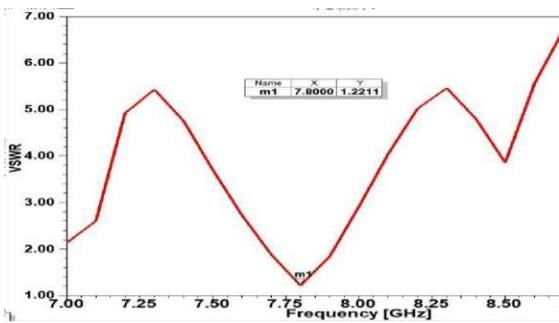
**Fig.5 VSWR with respect to Frequency.**
