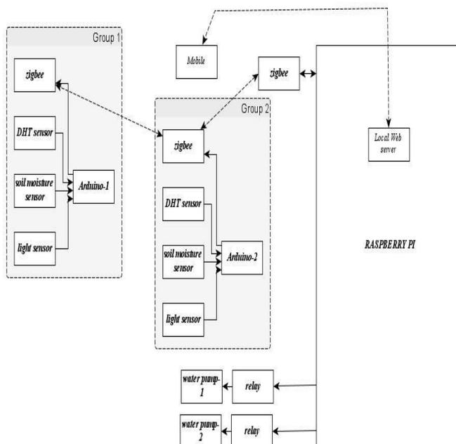
**Fig -1:** Block diagram of the proposed system
