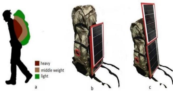
Fig- a) Distribution of weight on the backpack b) Prototype of the backpack(one solar panel active) c) Prototype of the backpack (two solar panels active)
