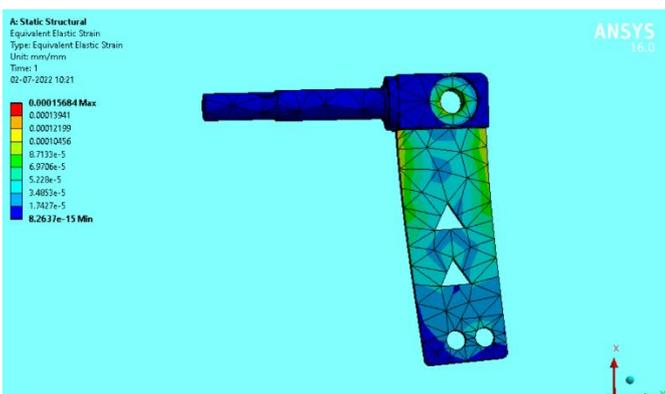
Fig -5b: Equivalent elastic strain of old stub arm
