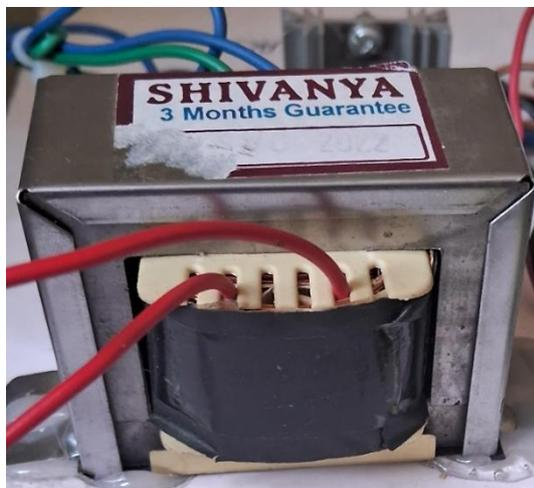
Figure 7: step-up transformer
