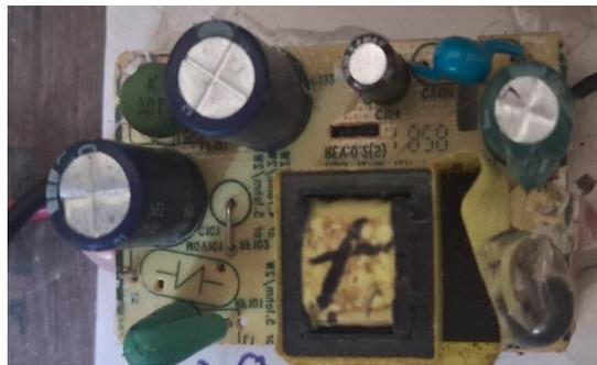
figure 4: AC-DC Converter
