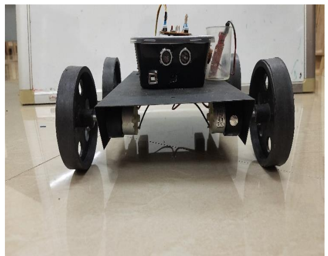
Figure 10: Back view of model with Ultrasonic and Programming port
