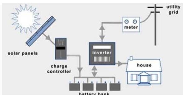
Figure 1. Block diagram of hybrid inverter
