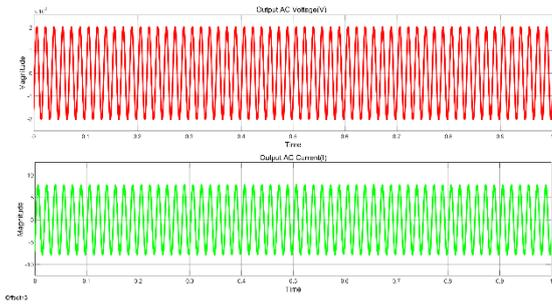
Figure 6. Output Waveform of AC Voltage and Current after filter
