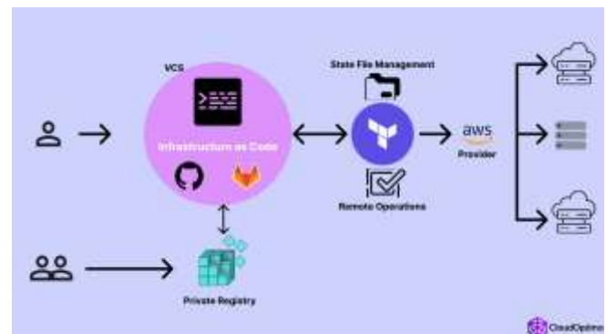
Fig. 1. Infrastructure provisioning workflow using Infrastructure as a Code (IaC) with Terraform.
