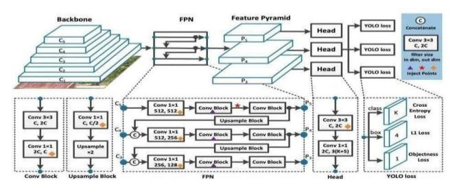
Fig4. YOLO V8 ARCHITECTURE
