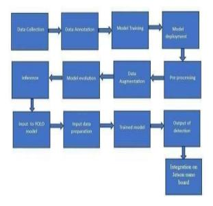
Fig2. Block diagram of safety vest detection using yolo v8
