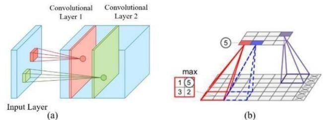
Fig. 6 (a) Process of convolution, (b) Process of pooling
