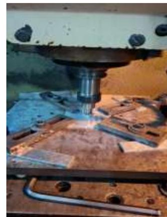
traverses along the joint line, transporting plasticised material from the leading to the trailing edge of the pin where it consolidates under shoulder forging pressure.
