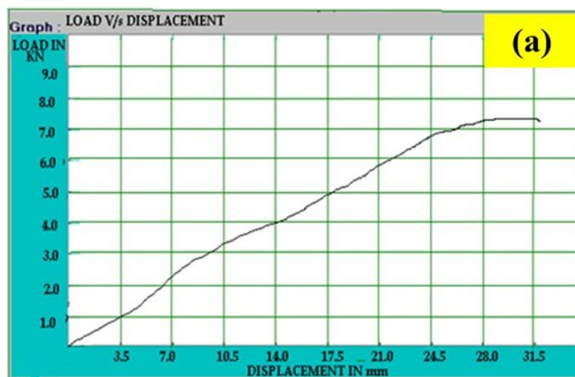
Fig 2.1 Graphical representations of Load (kN) V/s Displacement (mm) curve of Pure Aluminium.
