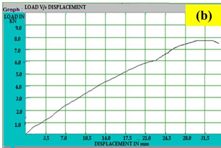
Fig 2.2 Graphical representations of Load (kN) V/s Displacement (mm) curve of Al + 2 Wt. % MWCNT.
