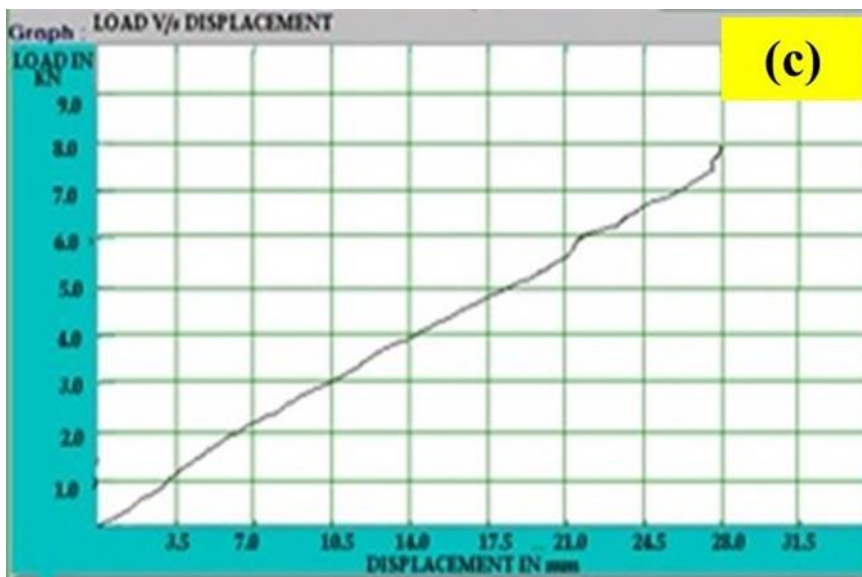
Fig 2.3 Graphical representations of Load (kN) V/s Displacement (mm) curve of Al + 2 Wt. % MWCNT+ 1 Wt. % fly ash.
