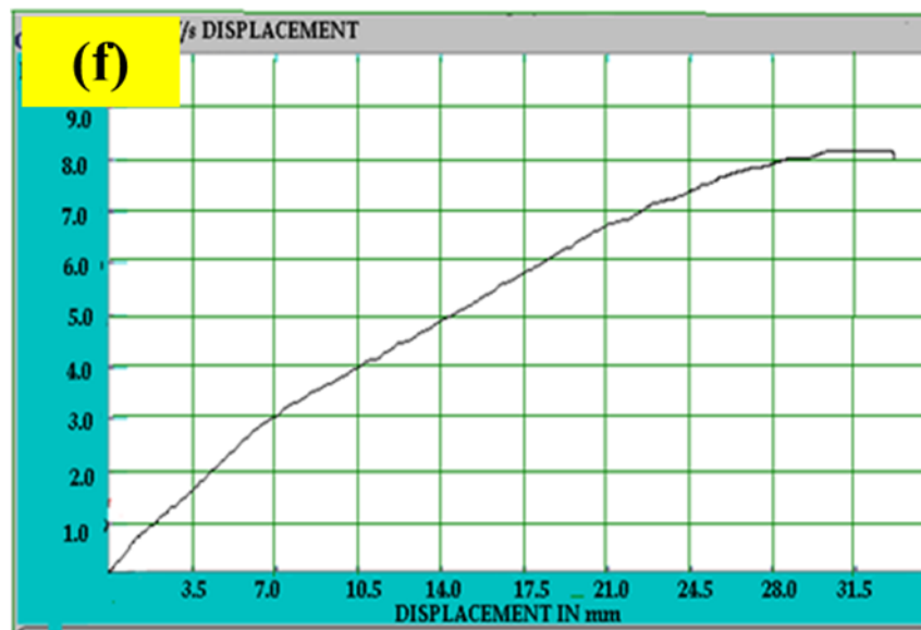
Fig 2.6 Graphical representations of Load (kN) V/s Displacement (mm) curve of Al + 2 Wt. % MWCNT+ 5 Wt. % fly ash.
