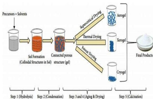
FIGURE 1: Schematic of different stages of sol-gel process: from precursor to aerogel [1-5].
