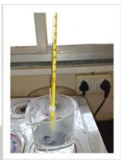
Fig 13 – Melting point test
