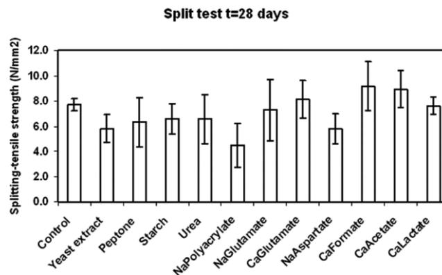
Figure 4. Splitting-tensile strength of organic compound-enriched (0.5% of cement weight) cement paste after 28 days curing.
