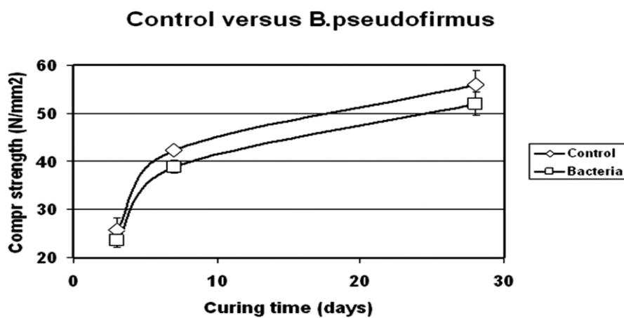
Figure 3. Compressive strength development of control and bacteria-added cement paste samples in time.
