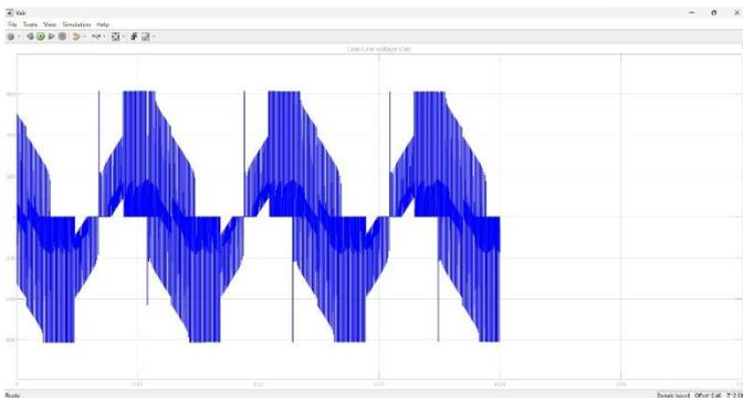
Fig 5 Line-to-Line Voltage of Inverter Output
