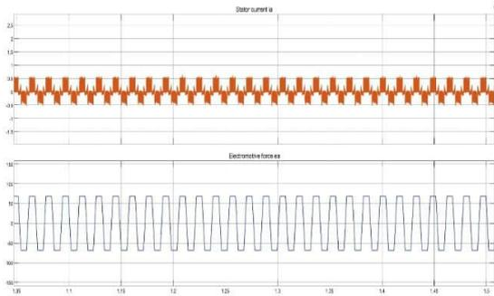
Fig 4 BLDC motor stator current and back EMF
