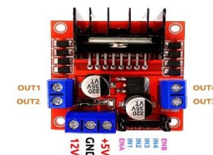
Fig 3.1.1 L298 Motor Driver
