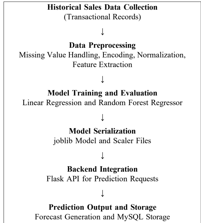
Fig. 2. Overall workflow of the sales projection system from raw data to prediction output.
