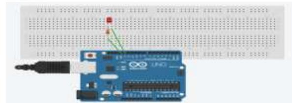
**Fig -13: LED blinking**
