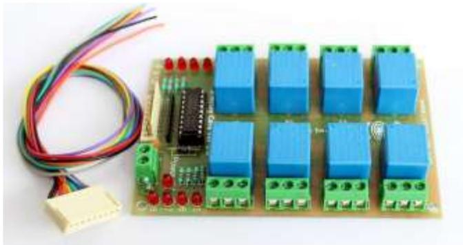
**Fig - 5.:** Relay board
