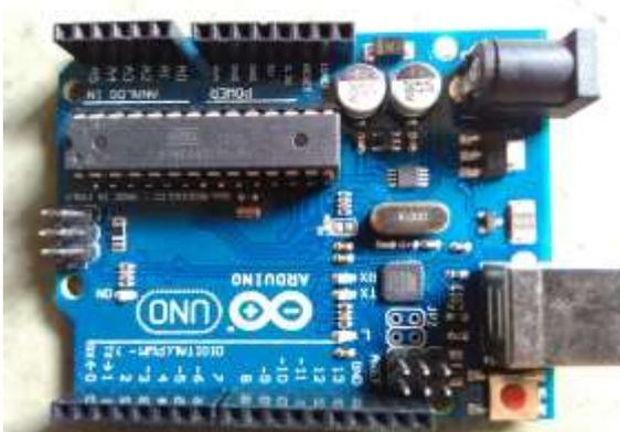
**Fig -16: ARDUINO AT mega 328**
