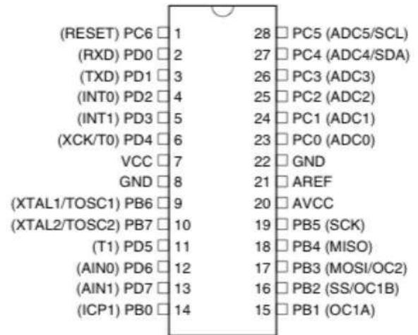
**Fig -17: Pin diagram of AT mega-328**
