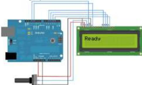
**Fig -14:** LCD interface
