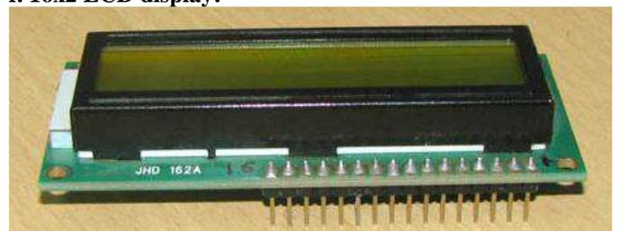
**Fig -9: 16x2 LCD display**
