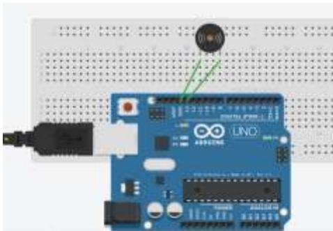
**Fig -15:** Buzzer interface
