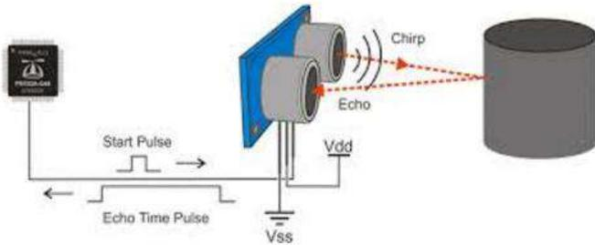
**Fig -11: Operation of ultrasonic sensor**
