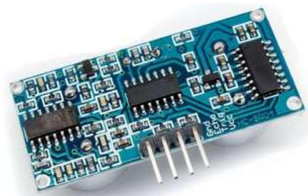
Fig -4: Ultrasonic Sensor Back Side
