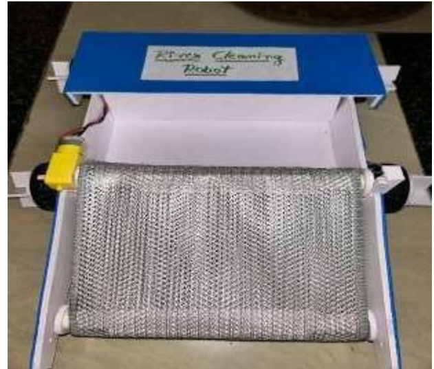
Fig 3: Complete model of river cleaning robot
