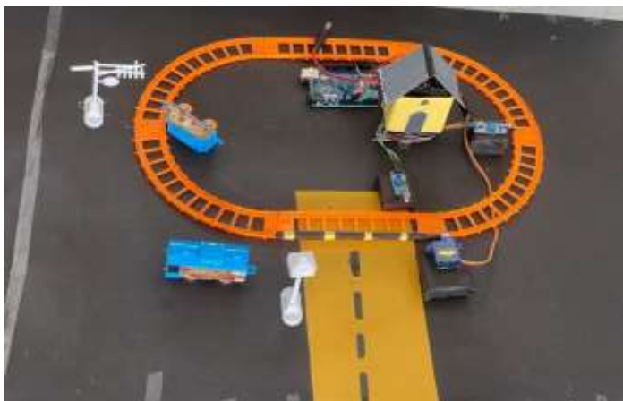
Fig. 2: Hardware Implementation of Automatic Railway Gate Control System Using Arduino
