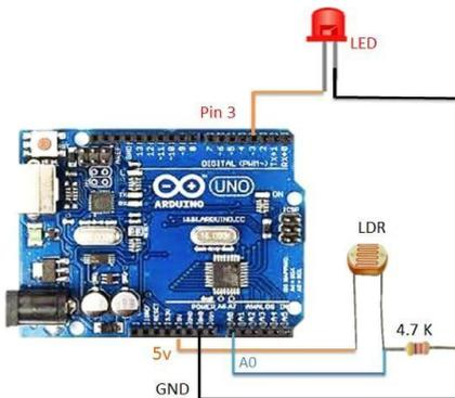
Light Detection using LDR and Arduino
