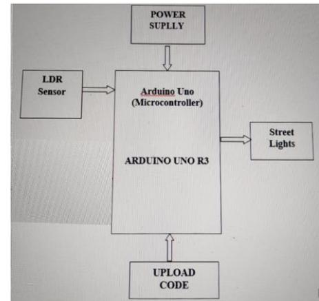
Figure 1. Block diagram interaction of components of automatic light controller
