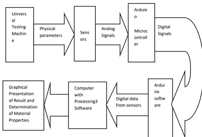
**Fig- 1** Block Diagram of Digital Universal Testing Machine
