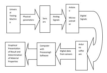
**Fig-1** Block Diagram of Digital Universal Testing Machine Figure 1 shows block diagram of digital universal testing machine presents development of existing hydraulic universal testing machine. Digital universal testing machine mainly consist of hydraulic analog universal testing machine, sensors, Arduino microcontroller, computer with Processing3 software.
