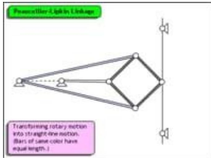
**Figure1.24** The Peaucellier Mechanism
