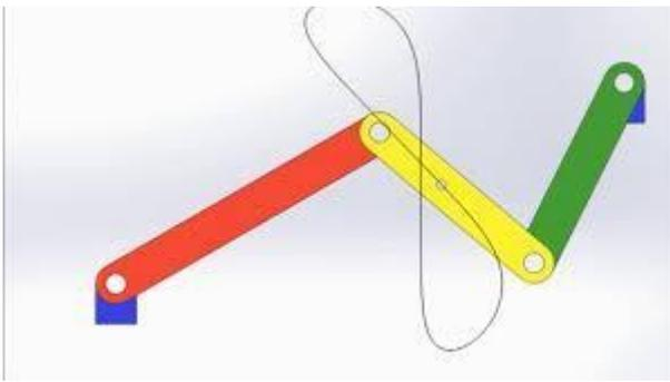
**Figure 1.21** The Watt Mechanism.
