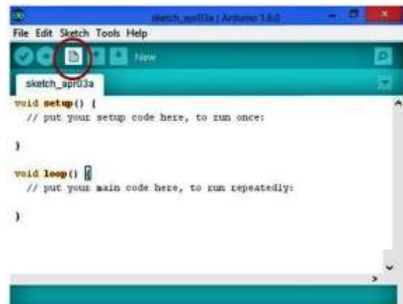
Figure-5: To create a new file in Arduino software
