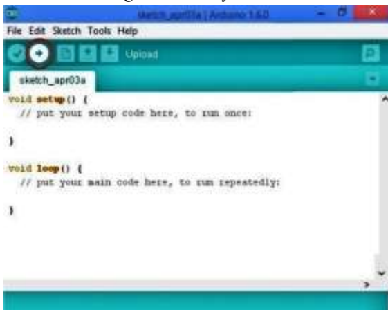
Figure-4: Upload in Arduino software
