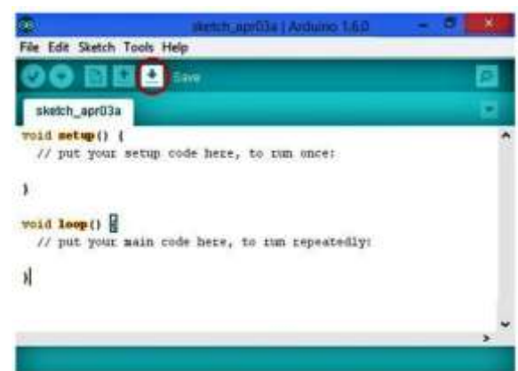
Figure-7: To save an new file in Arduino software
