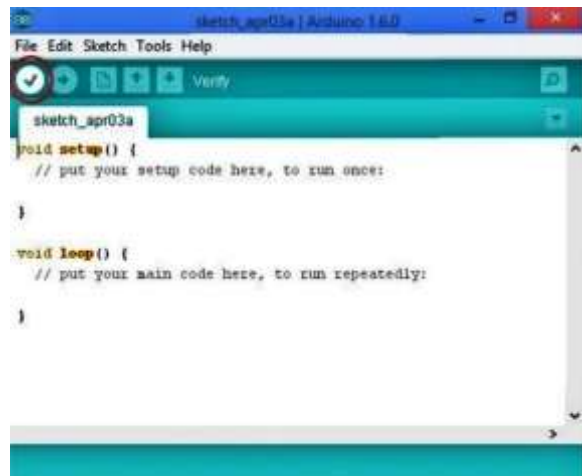
Figure-3: Verify in Arduino software
