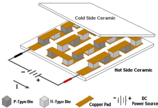
Internal construction of thermo- electric module
