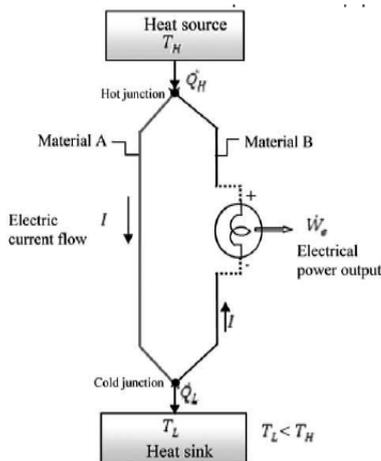
TEG consists of one hot side and one cold side. The hot side with higher temperature, will drive electrons in the n-type leg toward the cold side with lower temperature, which cross the metallic interconnect, and pass into the p-type leg, thus developing a current through the circuit. If temperature difference is kept constant, then the diffusion of charge carriers will form a constant heat current, hence a constant electrical current.
