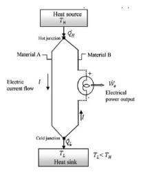
TEG consists of one hot side and one cold side. The hot side with higher temperature, will drive electrons in the n-type leg toward the cold side with lower temperature, which cross the metallic interconnect, and pass into the p-type leg, thus developing a current through the circuit.
