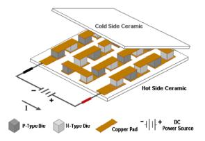
Internal construction of thermo- electric module
