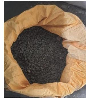
**Figure 4 :** Using Non-porous Aggregate with specific gravity 2.7 and size of 20mm check with flakiness index
