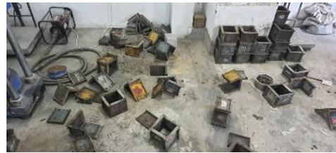
**Figure 3 :** Using mould of size 150x150x150mm for casting of cube
