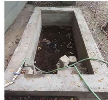
**Figure 5 :** Used curing tank for cube for 7 , 14 and 28 days simultaneously
