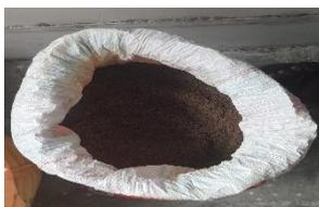
**Figure 2 :** Using Non-porous sand for the concrete mix size between 0.15mm – 4.75mm
