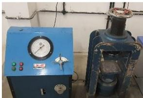
**Figure 1:** Compression Testing Machine (CTM)
