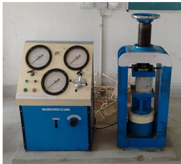
Fig 1. Compressive Strength Test Machine
