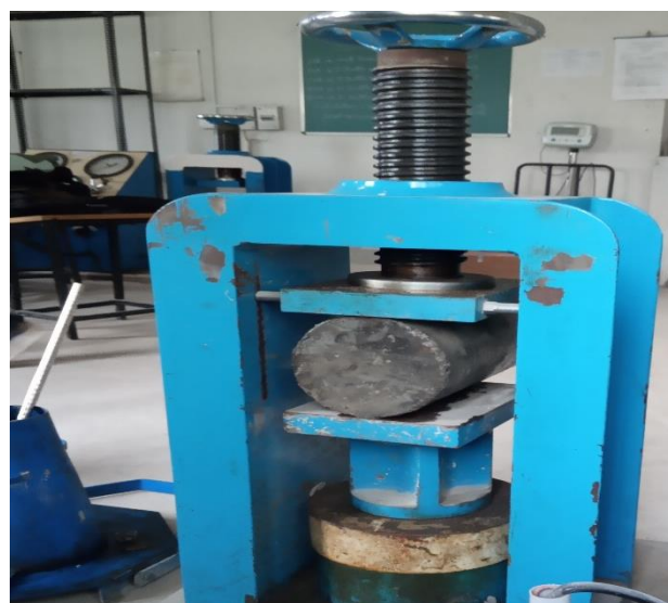
Fig 1. Split Tensile Strength Test Machine
