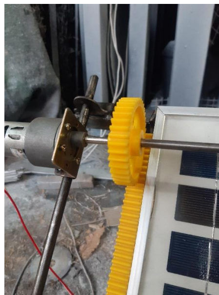
Figure.1.3: 12V DC motor with rack and pinion.
