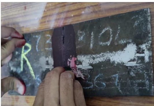
Figure 6.3: Removal of excess penetrant
