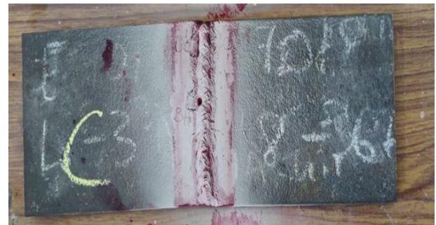
Figure 6.6: Inspecting on Cap face weld
