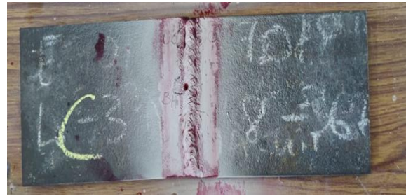
Figure 6.5: Defect on the weld area
