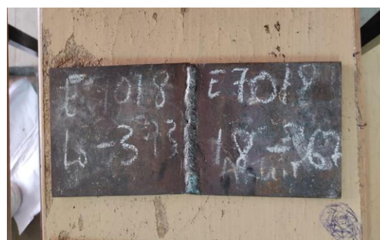
Figure 5: Welding done by E7018
