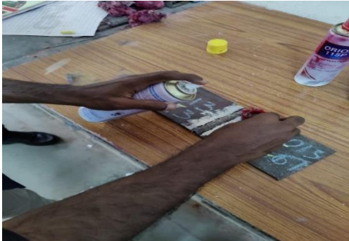
Figure 6.2: Applying Penetrant on weld area
