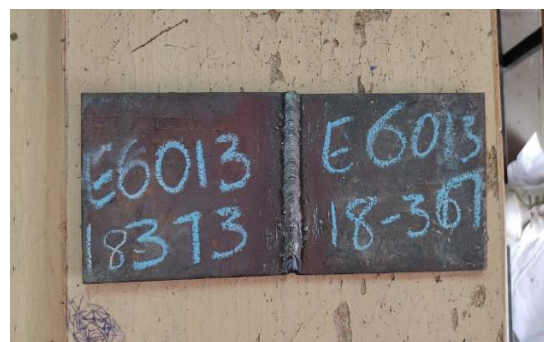
Figure 4: Welding done by E6013
