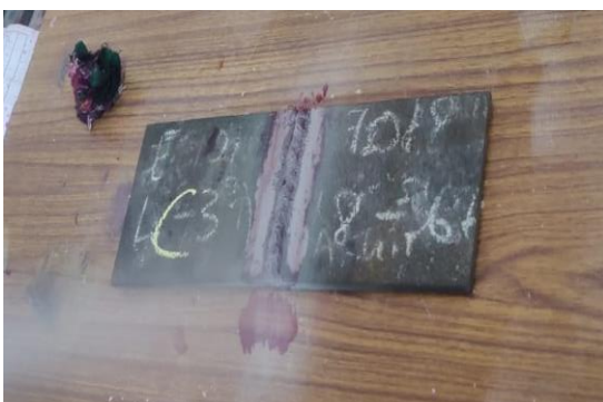
Figure 6.4: Developer applied on work piece
