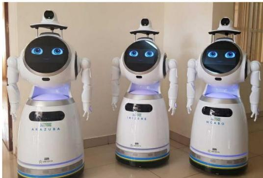
Figure 4.3.1: Thermal camera attached at the top.
