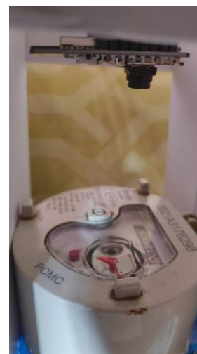
Fig. 5 ESP32-CAM Based Automated Water Meter System
