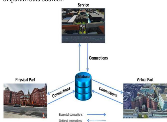
Figure 1. Predictive digital twin structures
