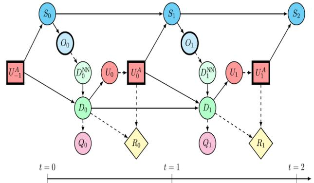
Figure 2. Dynamic decision network encoding the asset-twin coupled dynamical system
