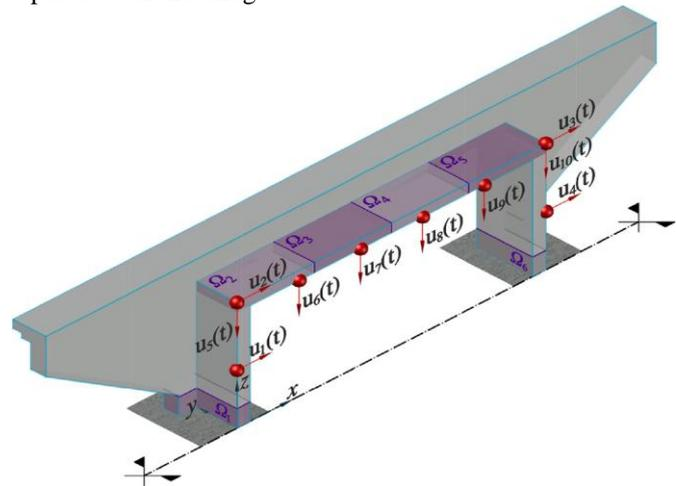
Figure 7. Railway bridge : details of synthetic recordings related to displacements  $u_1(t), \dots, u_{10}(t)$ , and predefined damage regions  $\Omega_1, \dots, \Omega_6$ .
